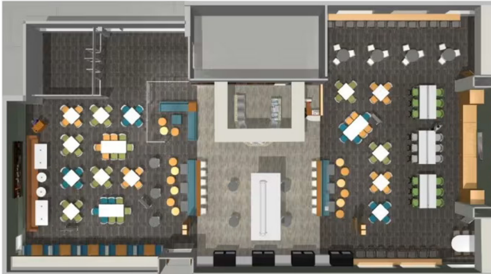
Reference layout. 136" dvLED video wall, 98" centerpiece display, 55" column displays, motorized projection.
