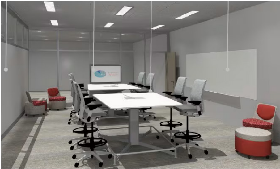
Reference layout: dual 98" LG displays + 75" DTEN D7 touch on the front wall, wall-to-wall whiteboard, split table with stool-height seating.
