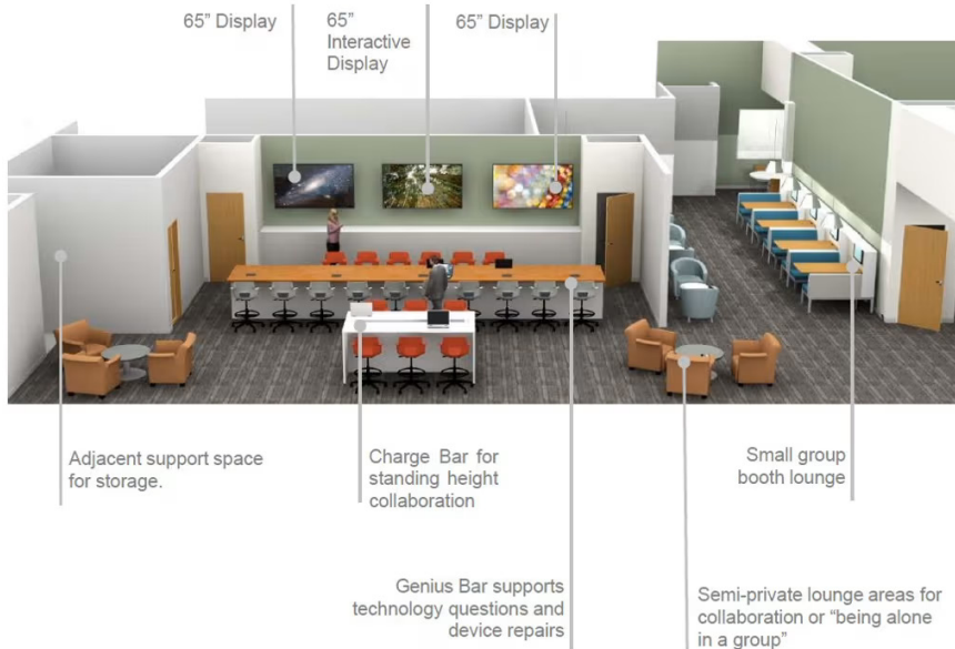
Reference layout: 65" Avocor touch flanked by 2x 65" LG displays, high-top tech bar, four booths with 43" displays, lounge seating.
