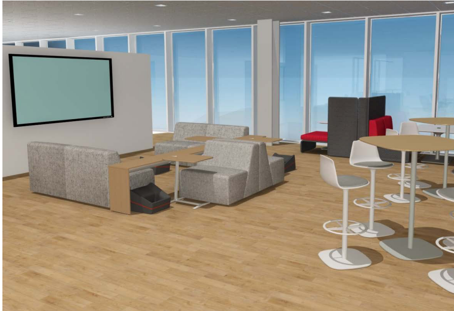
Reference layout. 85" primary, interactive 85" display and 138" DVLED display + mobile stand, with room presenter & audience cameras.
